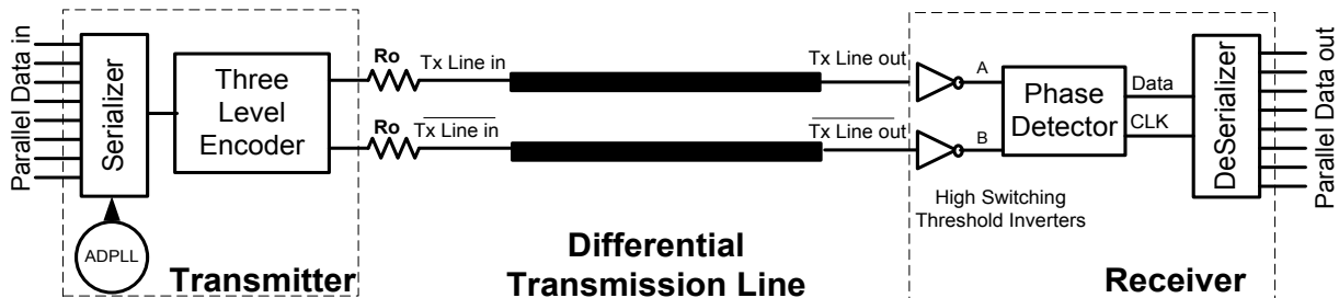
Figure 2.23 SerDes transceiver architecture for 3 level signaling preserving the DC level in scheme 2
